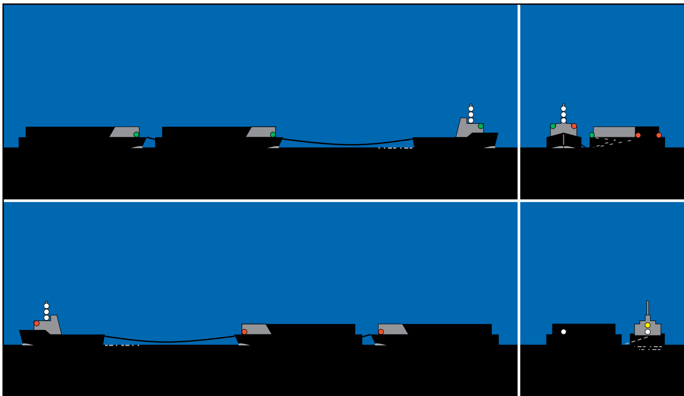
Vessel engaged in towing, where the length of tow is more than 200 metres, measured from stern of towing vessel to stern of tow, and the towing vessel is less than 50 metres in length.
