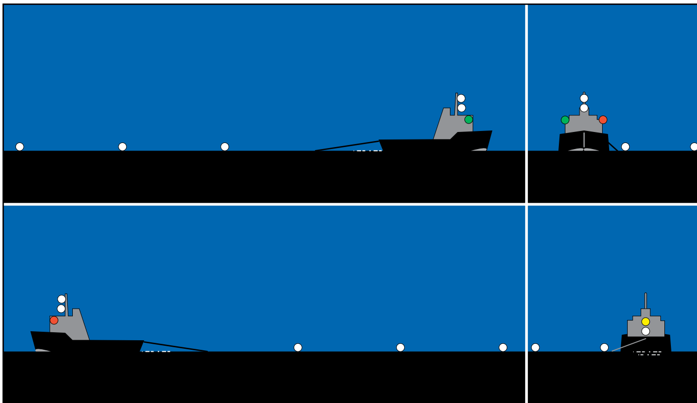
Vessel engaged in towing a log boom, where the length of tow is 200 metres or less, measured from stern of towing vessel to stern of tow, and the towing vessel is less than 50 metres in length.
