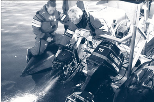
Water is expelled from cylinders
